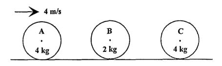
A is projected with a velocity of 4 m/s so as to collide directly with B. The coefficient of restitution for the collision is ½. Find the velocity of A and the velocity of B after this collision.
